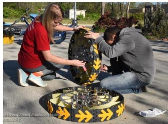
Experience: The steel construction worked well, however, the pre-tensioned leaf springs jumped out of their bracket from time to time and the tire was not rough enough and therefore offered little road grip. Added to this was the heavy weight, so the wheels proved to be somewhat impractical.
