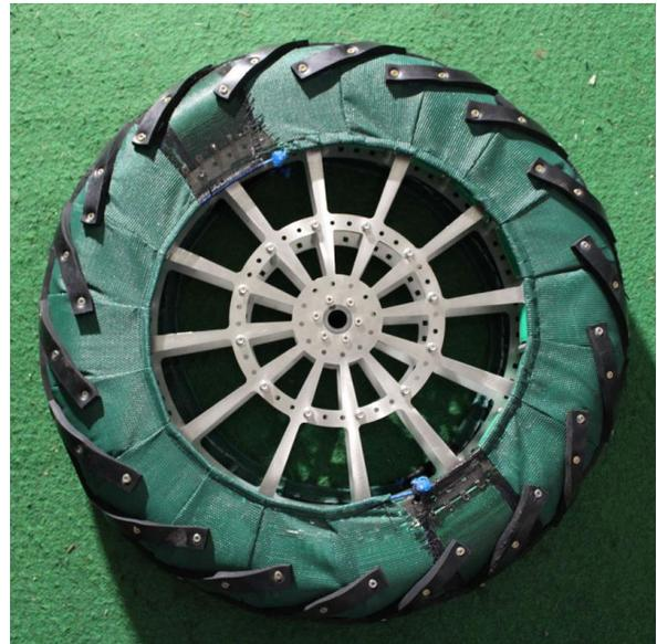
Self-resonance: The self-resonance is eliminated, because the number of wheel segments (19) is a prime number and all wheels are going to run differently.
